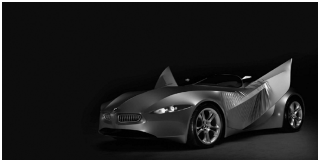
Figure 1-2 Picture of the prototype of the BMW GINA (Geometry and functions In 'N' Adaptations) 2001, a sports concept car entirely covered with a light fabric skin (Squatriglia, 2008). Source: BMW web page.
